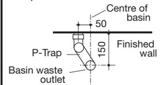
Fig 3 **Important: Accurate P-trap set-out for shroud is essential**
