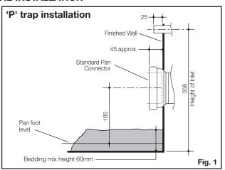
IMPORTANT: ALL DIMENSIONS ARE TO THE UNDERSIDE FOOT LEVEL OF THE PAN/CLOSET. IT IS IMPORTANT TO MAKE A HEIGHT ALLOWANCE FOR BEDDING.
