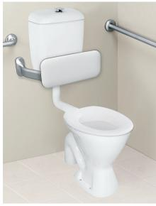
A pedestal type 6/3 litre dual flush Care Pan installation designed to provide a raised seat height of between 460-480mm for accessible applications &. The versatility of the Care Pan makes it ideal for use by both the ambulant people with disabilities and wheel-chair users including wheeled commode chairs.
