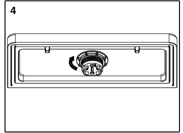
Hand tighten the nut fully.
