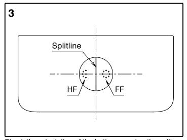
Check the orientation of the button ensuring the split line is perpendicular to the back wall.
